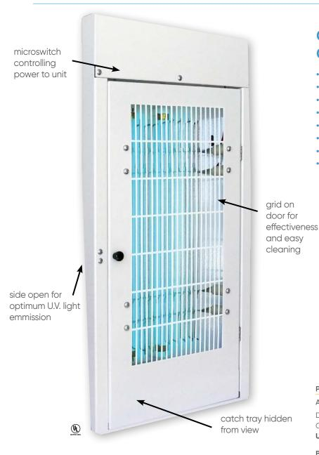
The **AG-963** Insect Electrocutor is designed for small areas where a compact light trap is the best choice. This corner/wall mount light trap is great for hallways and interior rooms where fly control is important. The AG-963 has a removable catch tray to contain dead insects for later evaluation, identification, and disposal. Install 3-6 feet high on the wall.
